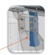
When installing the tension bracket, ensure to push the top side of the tension bracket behind the inner edge of the load bin to tension against.
